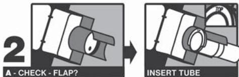
Check if your vehicle has a flap inside the filler neck. If there is a flap visible insert the tube into the filler neck, so that the sign TOP will be on highest position. Once the tube is inserted it enables the flap to stay open.
